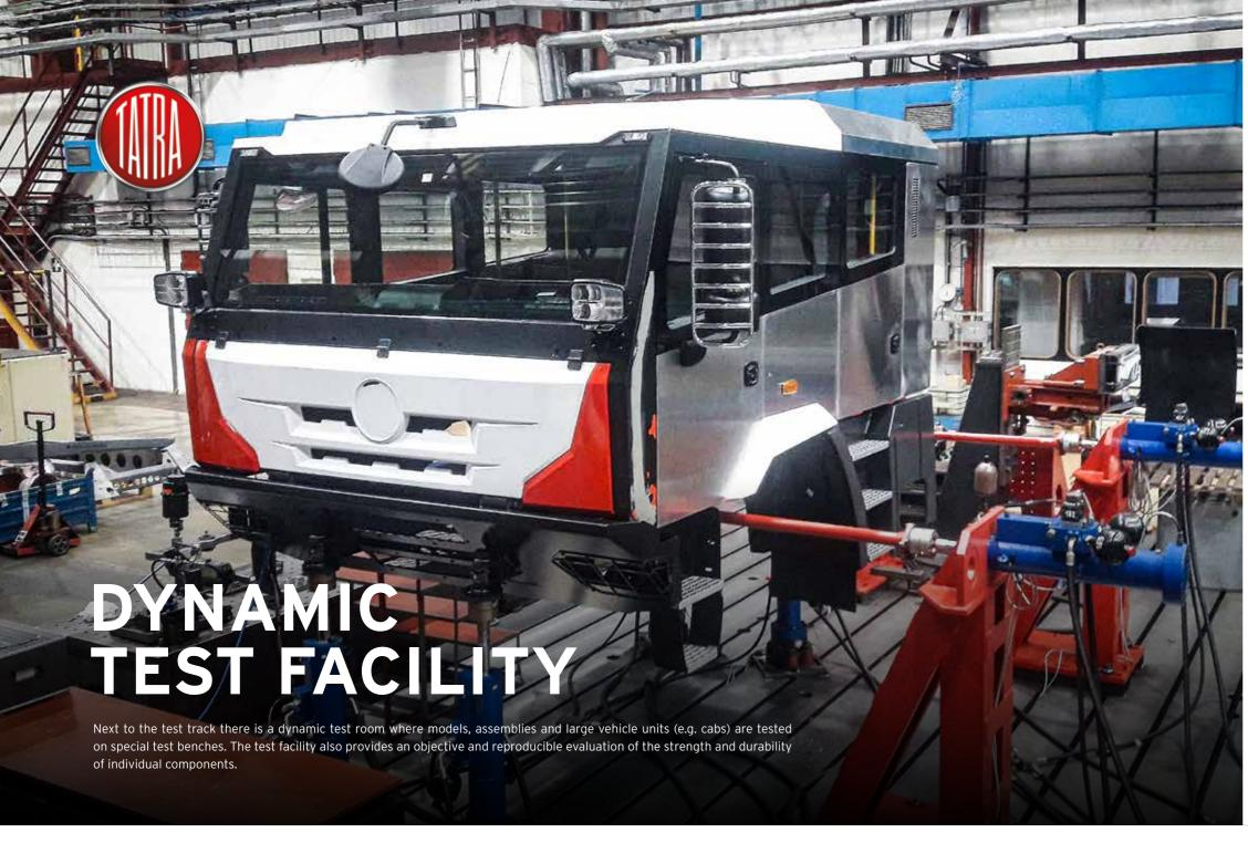
The principal purpose of the tests on the dynamic test benches is the repeatable loading of components identical (or very similar) to real operation. To this end, measurements are made in real operation or on special test centre roadways to obtain a load spectrum. This data is then used for accelerated condition tests.
