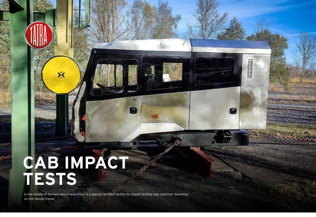
The test facility is equipped with a compressor for pneumatically operating the bumper clamps and special clamping devices for anchoring the cab test specimen to the base plate.
