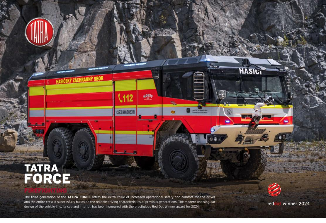
In addition to a major improvement in the existing TATRA FORCE concept with a low cab, engine over the front axle and a tunnel-free design, the third generation of the TATRA FORCE has expanded its portfolio to include variants with a front-mounted engine. As a new feature, the four-door cab provides above-average interior space and room for up to eight people.
