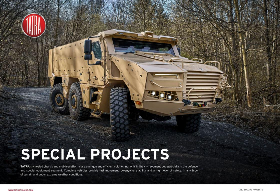
The exclusive ability to deliver unique added value to customers in the form of TATRA **MOBILITY** means the ability to provide a wheeled chassis or platform with the required number of axles, configured with an air-cooled or liquid-cooled inline six-cylinder engine, manual, automated or fully automatic transmission and cab preparation, or a complete superstructure for any customer project.
